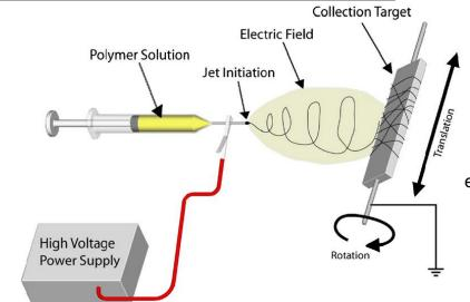
A schematic of the electrospinning process to illustrate the basic phenomena and process components
