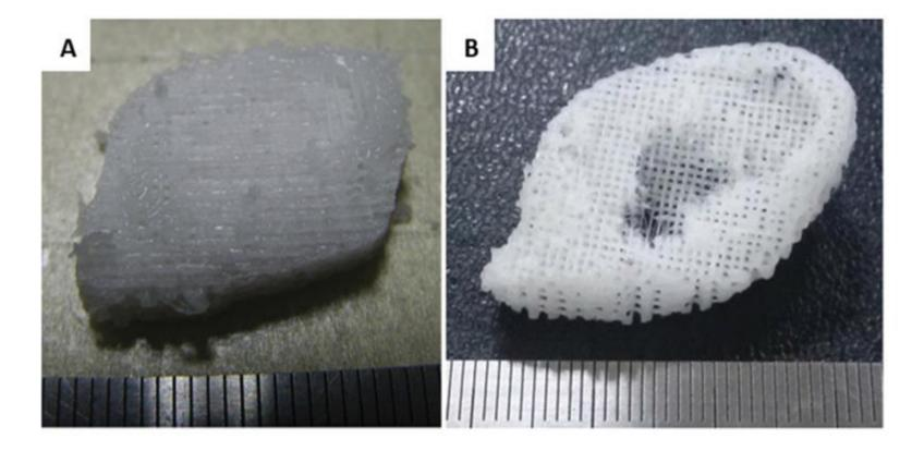
**Figure 7.** Ear-shaped scaffolds: Photographs of ear-shaped structures made from PCL using a PEG sacrificial layer (not shown) through a hybrid 3D printing system combining both inkjet printing and fused deposition modeling. A) back of ear scaffold, B) front of ear scaffold. Reproduced with permission.<sup>[27]</sup> Copyright 2014, IOP Publishing.
