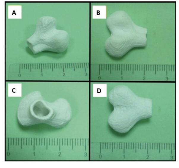
**Figure 12.** Bone scaffolds generated by SLS: A) Image of the scaffold, B) front view, C) top view, and D) back view of bone scaffold parts. Size is based on a centimeter ruler, with hatch marks indicating per millimeter. Reproduced with permission.<sup>[115]</sup> Copyright 2014, Elsevier.
