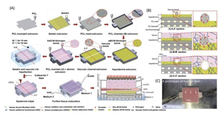
**Figure 17.** The 3D cell printing process for fabrication of 3D P/V full-thickness skin model. (**A**) Schematic diagram exhibiting the step-by-step fabrication process. (**B**) Sectional views provided from the aforementioned fabrication process. (**C**) A prototype of the fabricated skin construct. Reproduced from [249] with permission from John Wiley and Sons, 2018.
