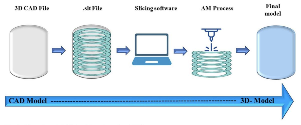
Fig. 1 Blueprint of Additive Manufacturing (AM)
