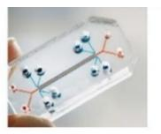
Microfluidic devices consisting of multi channels compatible with cell culturing which resembles the physical and physiological functions of a specific organ
