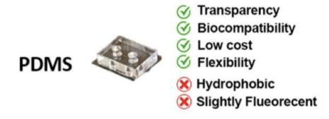
PDMS is the most common material used for the fabrication of microfluidic devices, and OOCs in particular. It is a silicon-based elastomer and has extremely advantageous properties, namely economic feasibility, transparency, flexibility, oxygen permeability, and biocompatibility. It also shows good compliance with various microfabrication techniques, such as soft lithography or molding.
