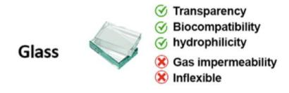
One of the oldest materials in the development of microfluidic devices is glass. In general, there are three types of glass used in this field: (i) soda lime, (ii) quartz, and (iii) borosilicate. They are a mixture of silicon dioxide (SiO2), the base material of glass, with other oxides, such as CaO and MgO.
