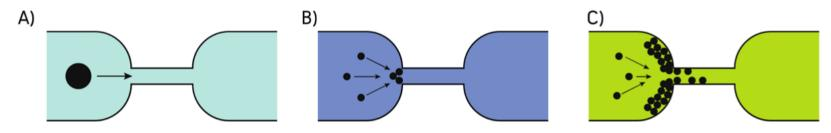
Figure 4. Clogging mechanisms: (A) sieving, (B) bridging, and (C) aggregation.
