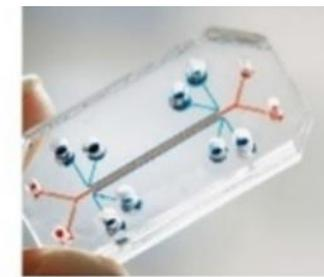
Microfluidic devices consisting of multi channels compatible with cell culturing which resembles the physical and physiological functions of a specific organ
