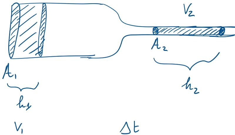
$$v_1 = v_2 = v \quad \text{fluido ideale}$$
