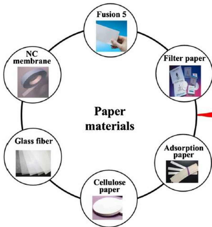
Fig. 1 Existing paper modification approaches for paper-based devices. Different paper materials, including Fusion 5, filter paper, chromatography paper, cellulose paper, Whatman® No.1 filter paper and NC membrane, are used for paper-based devices. Various reagents for paper-based detection are used.
