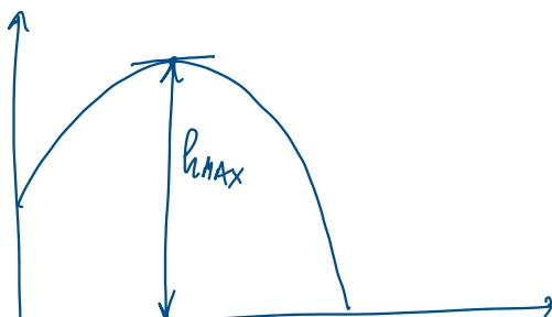
$$\begin{aligned} v_y &= 0 \\ t_{\max} &= \\ y(t_{\max}) &= h_{\max} \end{aligned}$$
