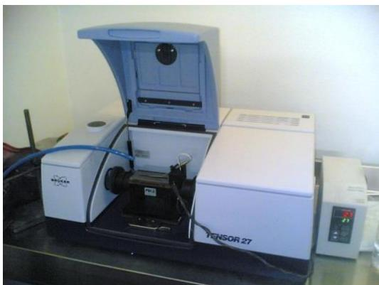
FTIR spectra acquired with Tensor 27<sup>TM</sup> FTIR (Bruker Optics, Milan, Italy), inteferometer Rocksolid<sup>TM</sup> and detector DigiTect<sup>TM</sup> with ATR. ATR (Specac Inc., Woodstock, GA, USA) had ZnSe crystal.
