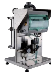
(RSLDE) Rapid Solid-Liquid Dynamic Extraction (Naviglio extractor)
