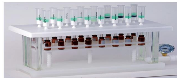
Schematic representation of SPE clean-up procedure
