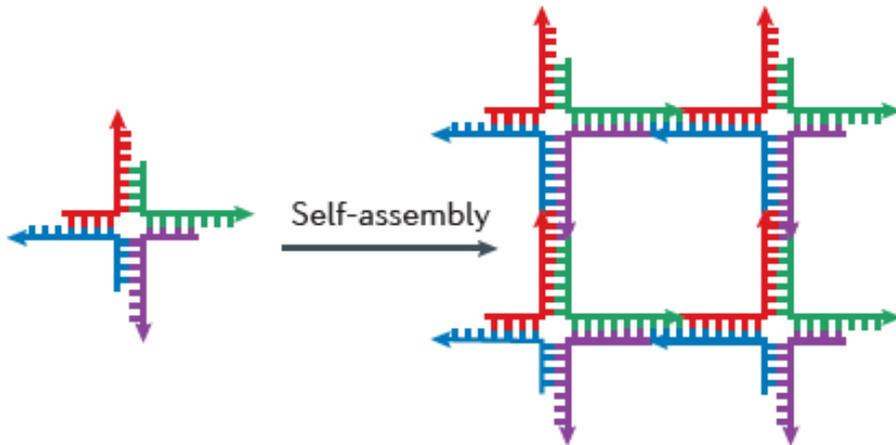
Branched junctions could be connected together by the base pairing of single-stranded overhangs, called sticky ends, into a 3D crystalline material
