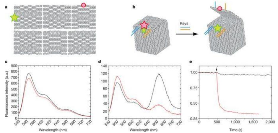
DNA box with a controllable lid that can be opened in the presence of externally supplied DNA 'keys'.
