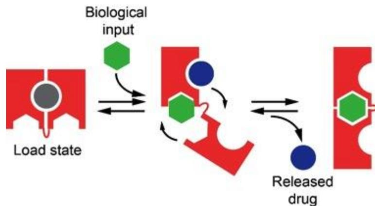
Rational design of a new class of DNA-based nanomachines *allosterically regulated* by specific biological targets, able to release a molecular cargo in a controlled fashion.
