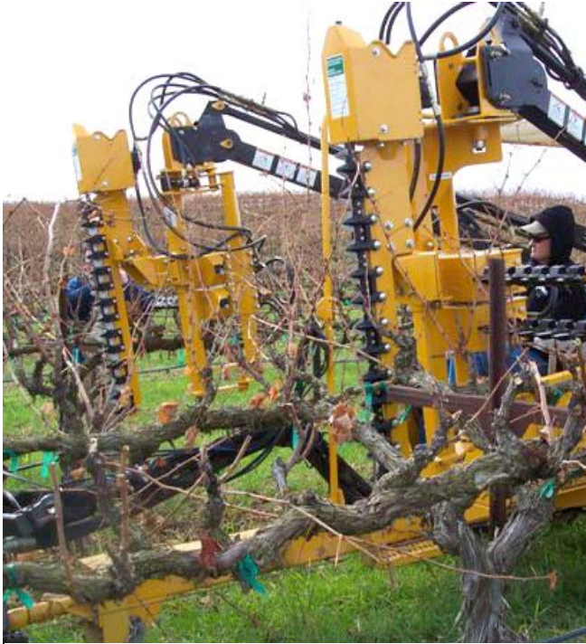
Figure 4. Shear pruning attachments on Korvan™ Vineyard System chassis shown working in Vitis vinifera vineyard at French Camp Vineyards, Santa Margarita, Calif. This configuration allows the tractor-pulled unit to prune facing sides of adjacent rows. (Photo courtesy of OXBO International Corp., Clear Lake, Wis.)
