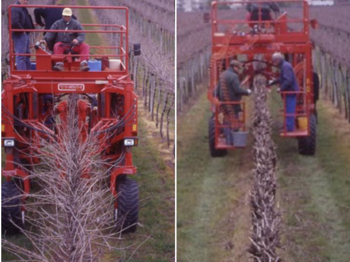
Figure 7. The TRINOVA during winter pruning of the MFC. It features two rear platforms equipped with power shears for rapid hand retouching.
