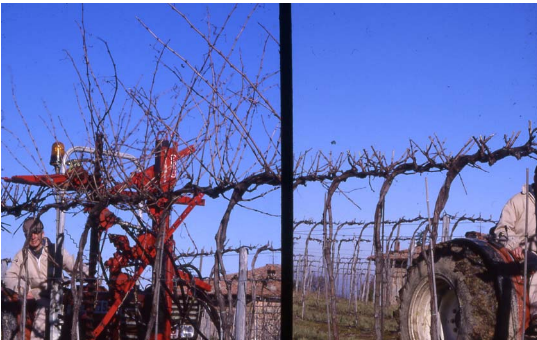
Figure 4. The Free Cordon (FC) during winter pruning with the TRIMMER unit.
