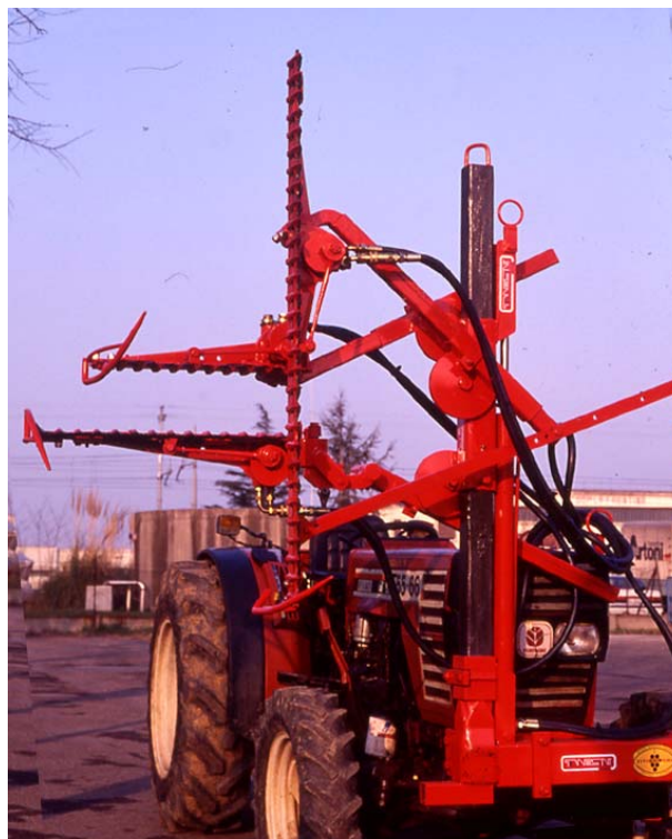
Figure 1. The TRIMMER machine. Incorporating all the upgrades since the original 1975 model, the unit has three adjustable cutters for winter-summer pruning of most systems, especially Spur-pruned Cordon, Double Curtain and Free Cordon. The current TRIMMER was designed by the University of Bologna's Chair of Viticulture in 1995 and built by the Faenza-based Tanesini company.
