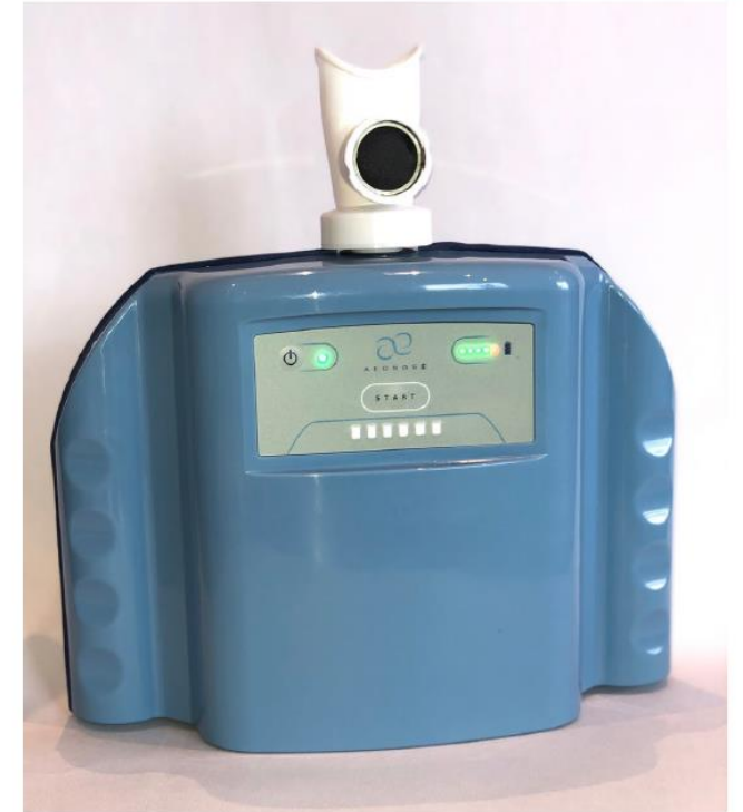
FIGURE 1 Electronic nose used in the study; the Aeonose (The eNose Company). Patients inhale through a carbon filter to prevent the entry of nonfiltered environmental air and breathe into the device through a disposable mouthpiece while wearing a nose clip
