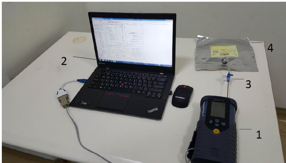
Figure S1. Experimental setup for the analysis of alveolar air consisting of a (1) E-nose, (2) computer, (3) three-way valve and (4) Tedlar bag.
