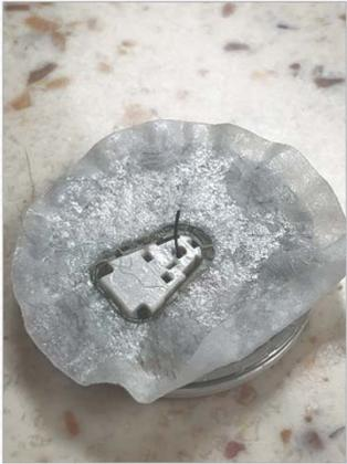
Figure 1. The adhesive side of a CGM sensor, after removal from a patient, showing the flexible polyurethane probe that stays in the interstitial space.
