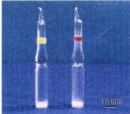
Figure 1. Vacuum-sealed ampoules with freeze-dried mouse spermatozoa. The white powder at the bottom of each ampoule is the dried CZB medium containing spermatozoa.
