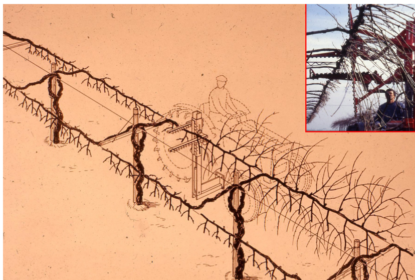
Fig. 3. Modified Geneva Double Curtain (GDC) training system to allow free cutting profiles around the cordon. In the inset a detail of cutter bar assembly during winter pruning.
