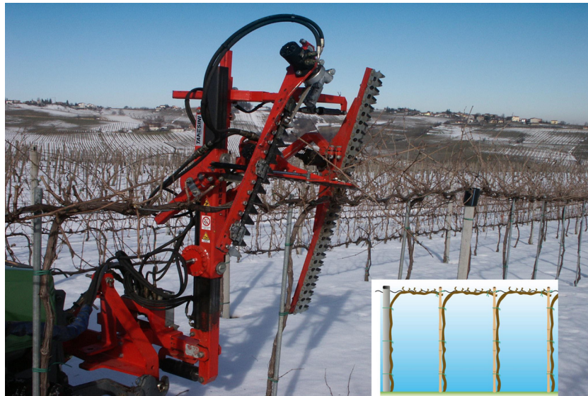
Fig. 5. A reversed C-cut profile during winter mechanical pruning on single high-wire trained vines. It is intuitive that having most of the pruning wood located above cordon greatly facilitates machine work and speed since manual cuts needed to remove ventral wood are kept to a minimum. The inset shows the frame and vine structure of the single high wire trellis.
