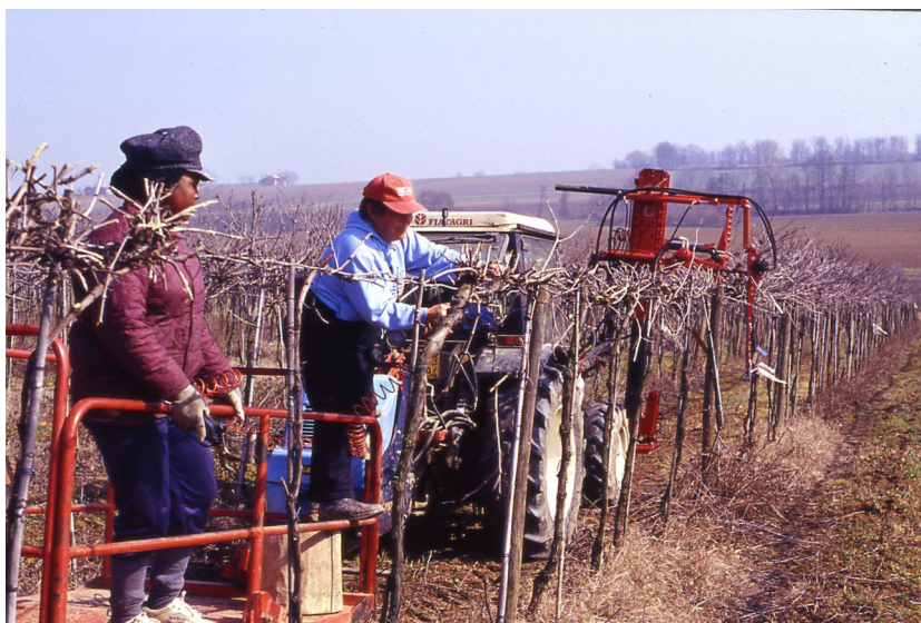
Fig. 6. A typical winter mechanical pruning set-up where machine pre-pruning is followed by hand finishing performed by two skilled workers using power shears.
