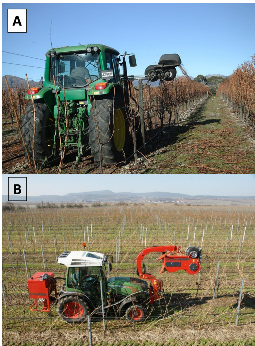
Fig. 12. (A) 'Vine stripper' machine showing two counter-rotating disks embarking canes in excess to convey them toward the shredding head. Cane debris are then interspersed in middle of row ( www.langlois.co-nz ). (B) The Viteco ® cane pruner (B, www.ero-binger.it ) operating on a vine row.
